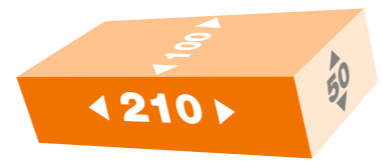
WF Waalformat 210 x 100 x 50 mm
